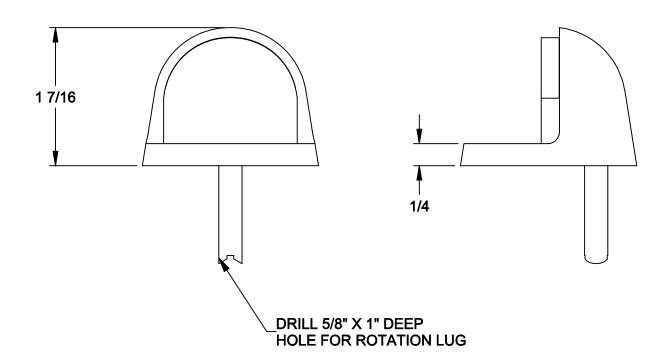
**FASTENERS PROVIDED:** 1/4-20 X 1" FH, PH, MS #14 X 1-1/2" FH, PH, SMS
