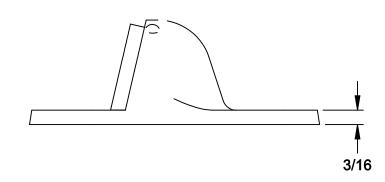
SUPPLIED WITH: TWO (2) 1/4-20 X 7/8 ANCHOR, 2 TWO (2) #14 X 1-1/4 PLASTIC BANTUMS, TWO (2) #14 X 1-1/2 FLAT HEAD, PHILLIPS DRIVE WOOD SCREWS, TWO (2) 1/4-20 X 1 UNDERCUT FLAT HEAD, PHILLIPS DRIVE MACHINE SCREWS AND TWO (2) 1/4-20 X 1 FLAT HEAD, TORX DRIVE MACHINE SCREWS.
